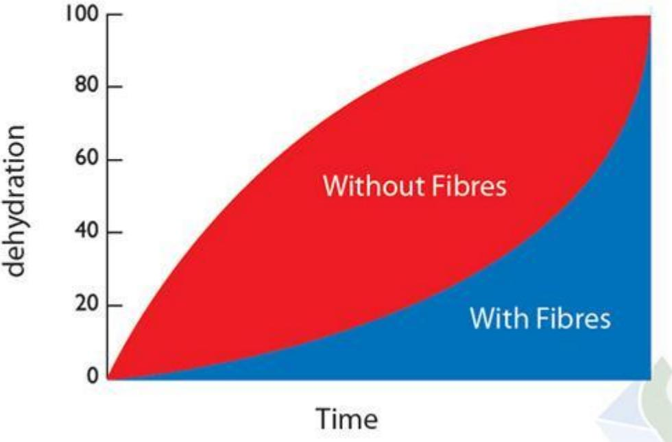
NYLON RC fibres added to the concrete mix will reduce the incidence of plastic shrinkage cracking by up to 86%.
